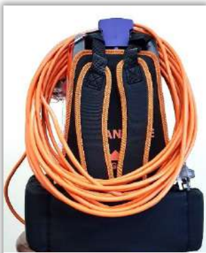
1. Loop the extension cord by gathering it from the machine end and drape it over the frame.
