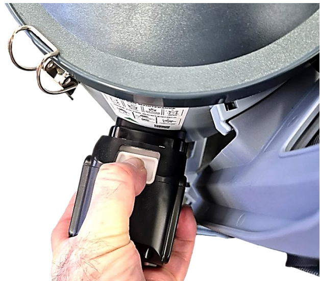
Fig 2. Releasing the battery from the Battery Holder
